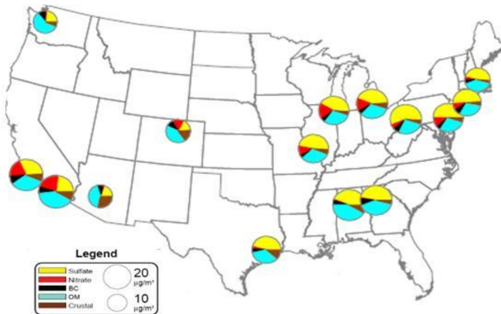
Figure B.3. Regional chemical composition of PM 2.5 aerosols -- composition of PM 2.5 for 15 selected urban areas in the United States. Annual average PM 2.5 concentrations ( \mu\text{g}/\text{m}^3 ) are presented, the circle size representing the magnitude of PM 2.5 mass.
