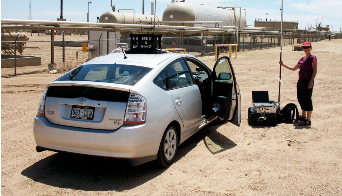
CIRES scientist Gabrielle Petron uses a specially equipped Toyota Prius to study air pollution. Photo courtesy Adam Hirsch
