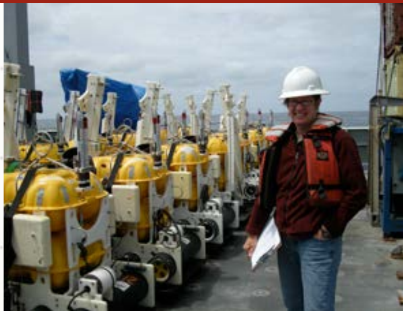
Sheehan in the South Pacific with ocean-bottom seismometers. These devices record Earth’s tremors in ocean locations.
