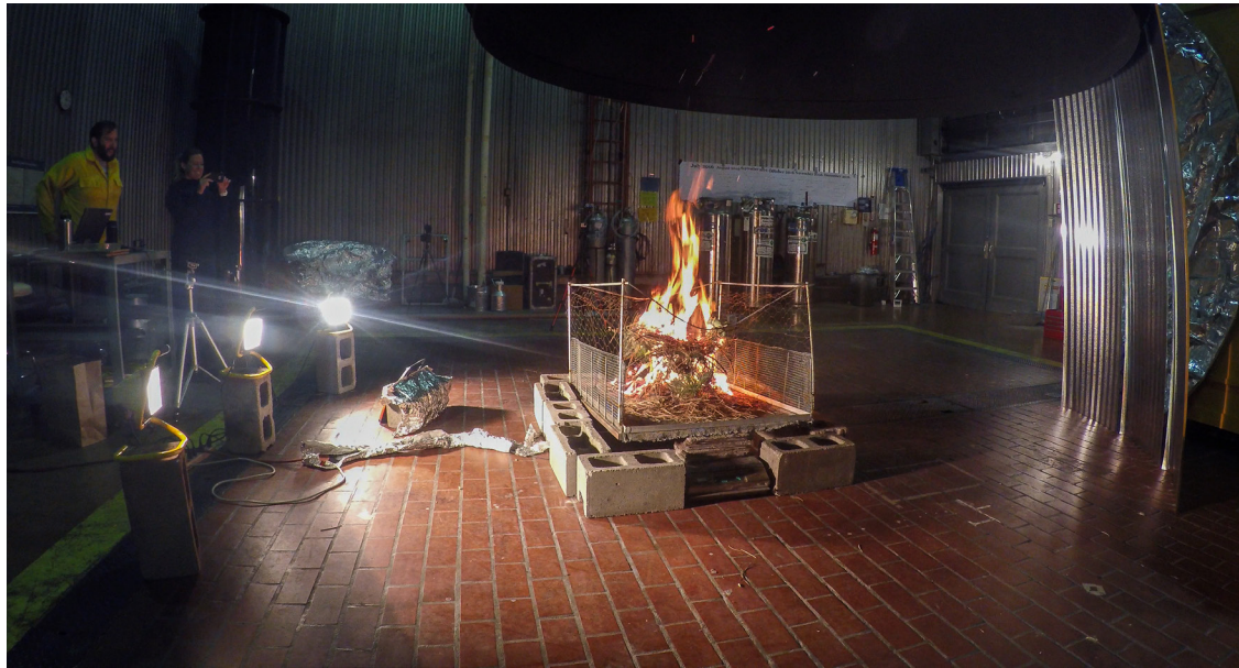
CIRES and NOAA scientists burned more than 100 fires made from various fuels found in the West, and sampled the emissions continuously with state-of-the-art instruments. Photo: Henry Worobec/ University of Montana
