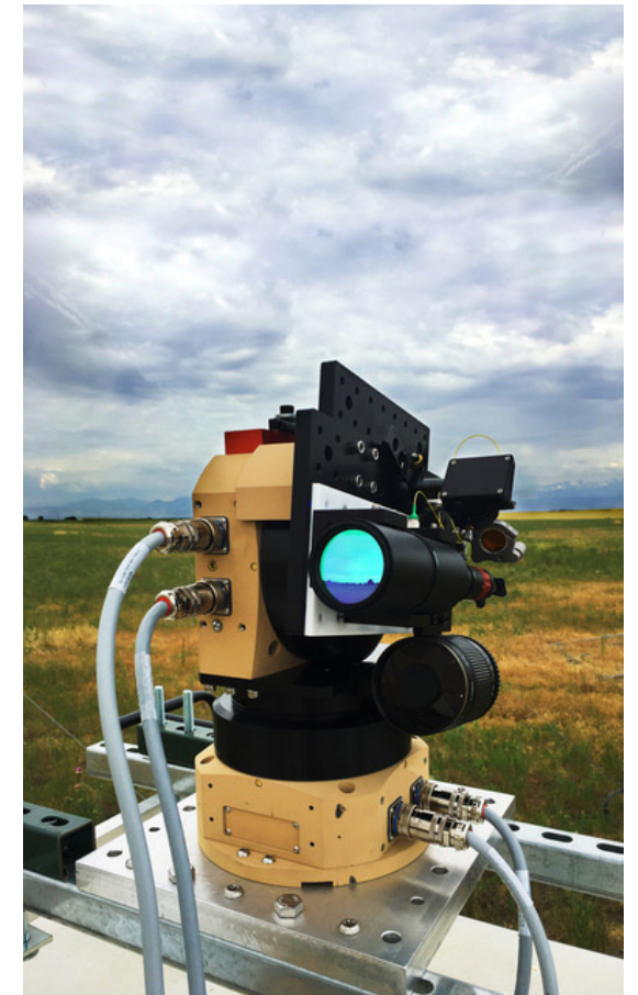
Dual frequency comb spectrometer observing system set up in the field. Photo: Caroline Alden/CIRES
