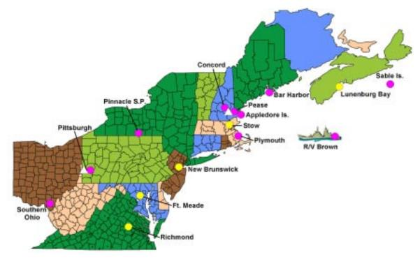
**Figure 29.** Proposed NEAQS-ITCT 2004 profiler network. Pink circles denote NOAA wind profilers, yellow circles denote cooperative agency wind profilers, and white triangles denote vertically-pointing unattended lidars. The full set of instrumentation on *Ronald H. Brown* is listed in a previous section.
