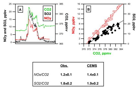
**Figure 2.** (A) An 18-km horizontal segment of NO<sub>y</sub>, SO<sub>2</sub>, and CO<sub>2</sub> data downwind of the Limestone power plant in east Texas on July 10, 2000. (B) Two-sided regression fits to data from (A). The table compares the derived emissions ratios to reported values using data from the continuous emission monitoring system (CEMS) installed at the plant.
