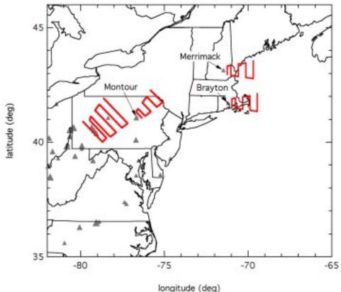
**Figure 20.** Potential flight tracks to study power plant plumes in New England (Merrimack, NH and Brayton, MA) and Pennsylvania (Montour, Homer City, Conemaugh, Keystone, PA) under a 5 m/s wind from the west and southwest respectively. The last transect shown is 144 km downwind from the power plants which for a nominal wind speed of 5 m/s corresponds to a plume age of 8 hours. Shown as grey triangles are the locations of major NO<sub>x</sub> point sources.
