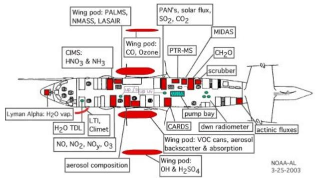
Figure 17: Proposed instrument layout for NOAA WP-3D Orion aircraft.
