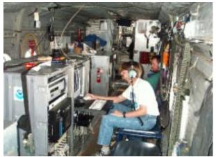
**Figure 22:** Airborne ozone and aerosol lidar deployed in NOAA-chartered de Havilland Caribou.
