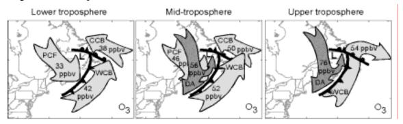
**Figure 3.** Median ozone mixing ratios (ppbv) associated with the various airstreams of midlatitude cyclones: warm conveyor belt (WCB), cold conveyor belt (CCB), post cold front airstream (PCF), and the dry airstream (DA). Measurements made during late summer, 1997, by the NOAA WP-3D aircraft during the NARE'97 experiment [*Cooper et al.*, 2002].
