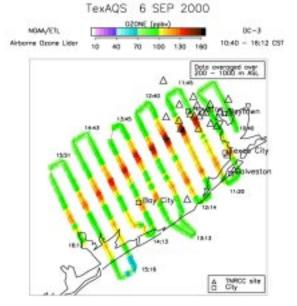
**Figure 23:** Flight track of lidar plume tracking measurements obtained during the Houston experiment. Ozone values are averaged over the layer between 200 and 1000 m AGL
