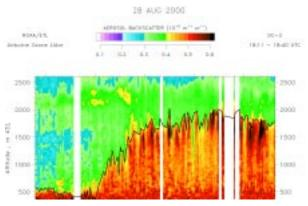
**Figure 24:** Vertical profile of lidar-observed aerosol backscatter showing a sharp change in mixing layer height at the Gulf of Mexico coast.
