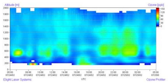
**Figure 27.** 24-hour time height cross section of ozone mixing ratio observed with the unattended ozone lidar at Pinnacles State Park on 24 July 2002.
