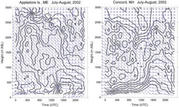
**Figure 26.** Diurnally-averaged wind profiles from the boundary-layer wind profilers deployed at Appledore Island, ME and Concord, NH during NEAQS 2002. Wind barbs show the vector-averaged wind direction. Contours (m s<sup>-1</sup>) indicate scalar wind speed.
