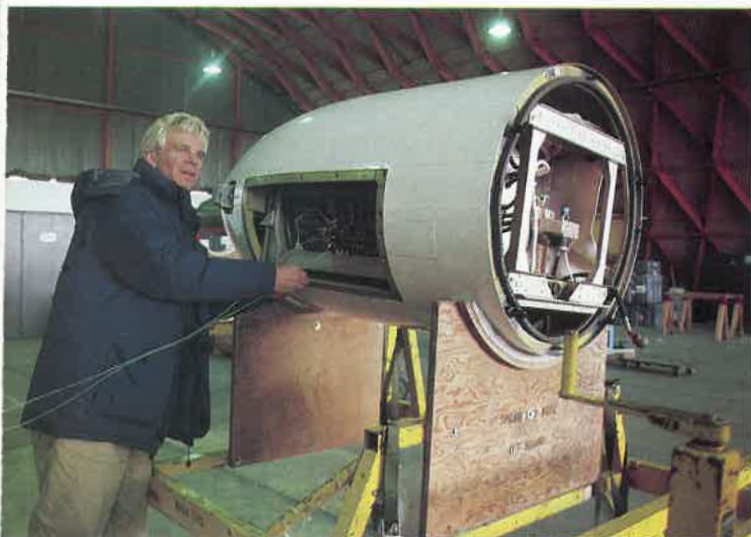
After ER-2 lands, Anderson connects pod experiment to his computer to copy out data collected in flight.
