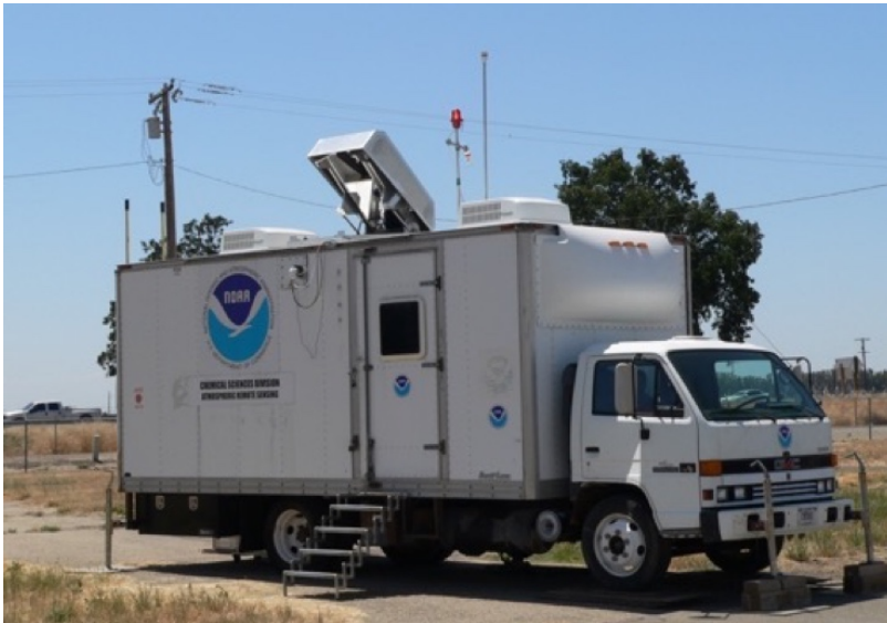
16 17 18 Figure 3. (Left) TOPAZ lidar truck parked at the Visalia Municipal Airport (VMA). The 2B 19 sampling mast can be seen to the right of the scanning mirror and warning light. Note the traffic 20 on CA-99 in the background. (Right) Composite vertical O 3 profile showing the altitude segments 21 derived from each of the slant profiles.
