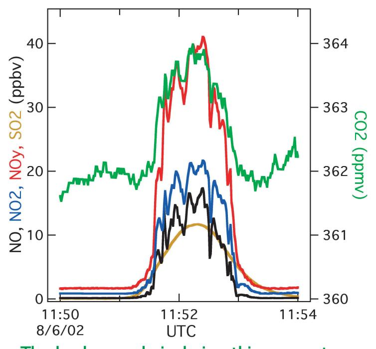
The background air during this encounter was relatively clean, so the plume from the ship exhaust stands out clearly. The data above are 1 second measurements of NO, NO<sub>2</sub>, NO<sub>y</sub>, SO<sub>2</sub>, and CO<sub>2</sub>, timeshifted for coincidence. As expected for fresh emissions, the ratio  $NO_x/NO_y$  is close to one. The fine structure in the data correlate well for all measurements except  $SO_2$ , which is due to slower instrument response.
