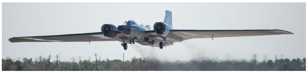
The WB-57 is a two-crewmember, high-altitude research aircraft that can reach altitudes of over 60,000 feet. http://jsc-aircraft-ops.jsc.nasa.gov/wb57/
