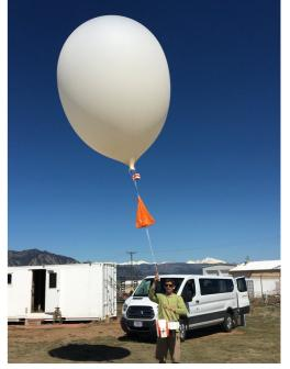
Helium-filled balloons carry sondes that relay data on pressure, temperature, ozone, humidity and particles. The balloon rises for 2 hours and bursts at 115,000 feet.
